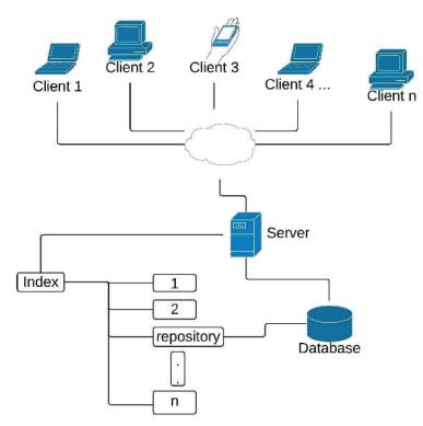
Figure 1. Client-server communication diagram. *Source:* Own elaboration based on Benito (2019, p. 41).
