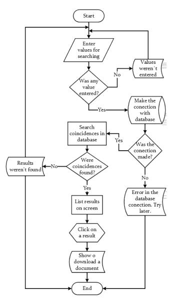
Figure 2. Repository flow diagram. Source: Own elaboration based on Benito (2019, p. 42).
